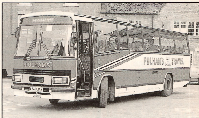
The three piece screen and twin leaf doors of a Paramount 3200 Express bodied Leyland Tiger at the Bourton terminal of the main Cheltenham service.
